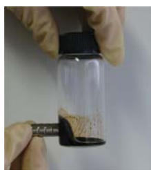
Movement of ferromagnetic fluid toward a small magnet
