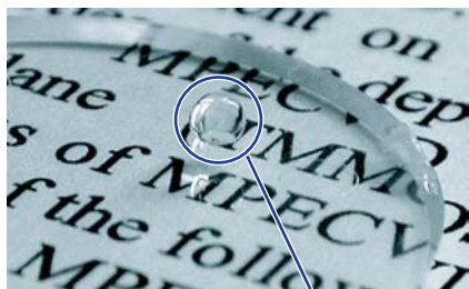
Waterdrop on the glass (surface is processed of UWR layer)
